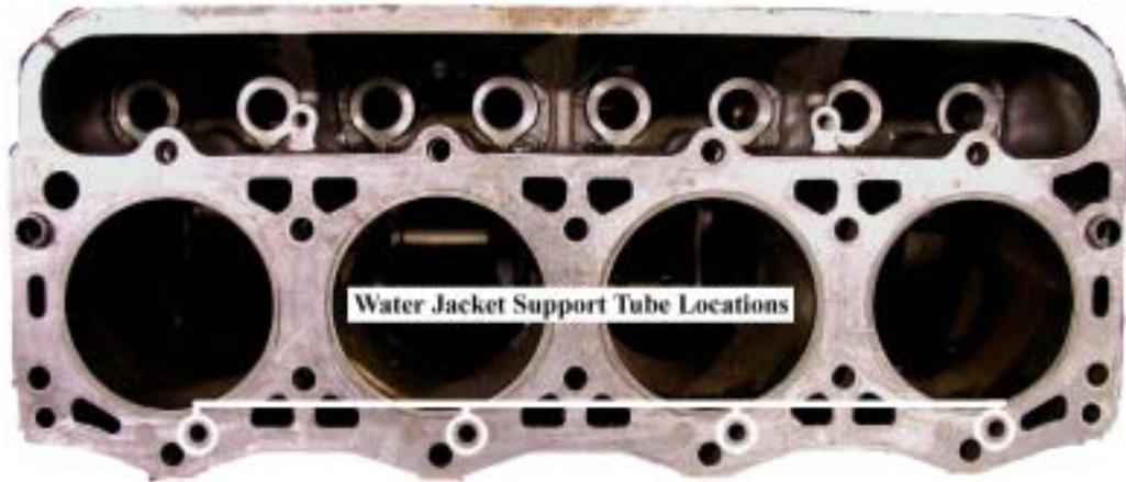
3. Using a 0.375" diameter reamer, ream the water jacket holes per **figure 2**. There are 4 per side and 8 total.
