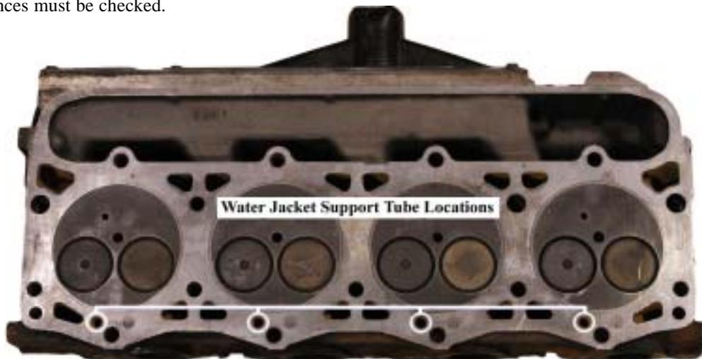
4. With the head surface clean and dowels removed, machine head per drawing **HYP-095**.
